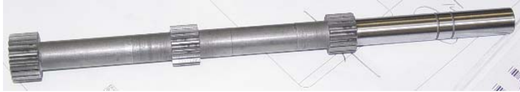
Figure 9 – The Finished Input Shaft
